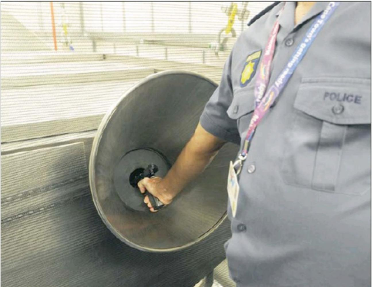
Pictured above: **BALLISTIC TESTING:** Lieutenant-Colonel Keith Rance fires a pistol in the testing room. After rounds are fired safely into the contraption, it spews the bullets and cartridge cases out at one end and sucks in water as part of a self-sustaining system. Test results are then analysed in a high-tech computer room. *Pictures: MICHAEL WALKER*
